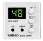
In-wall microphone module for paging for Mondo MTV816C, MTA816, MTA816S central unit
