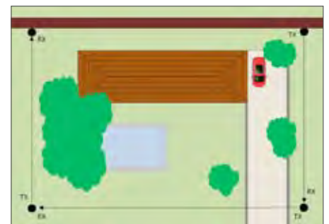
Solution with terminal and bi-directional columns
