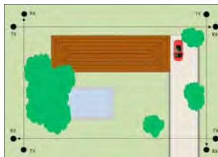
Solution with terminal columns
